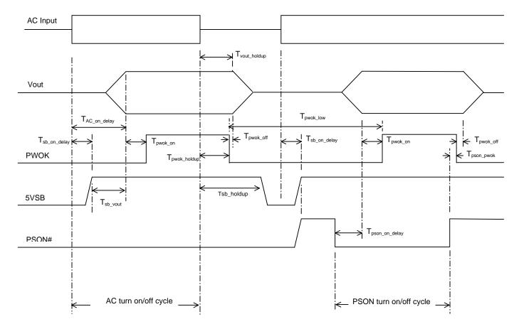
Figure 5: Turn On/Off Timing (Signal Power Supply)
